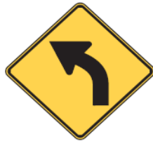
Figure 2C-1. Horizontal Alignment Signs and Plaques
