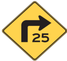
Figure 2C-1. Horizontal Alignment Signs and Plaques
